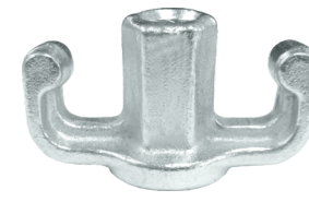
FORGED WING NUT Material : EN - 8 Weight : 0.350 kg. Working Load : 90 KN
