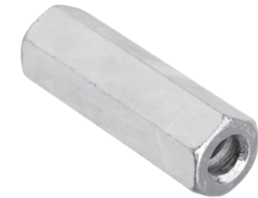
TIE BAR CONNECTOR Material : Mild Steel Size : 100 / 105 mm Weight : 0.450 / 0.472 kg.
