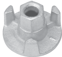
THREE WING ANCHOR NUT (70MM) Material : SG Iron Size : 70mm Weight : 0.460 KG Working Load : 90 KN
