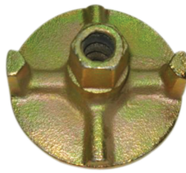
TWO WING ANCHOR NUT Material : SG Iron Size : Ø 70 / 100mm Weight : 0.400/0.590 KG Working Load : 90 KN
