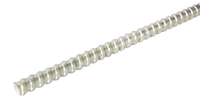
COLD ROLLED TIE ROD Material : EN - 8 / MS Size : Ø 15mm, upto 6mtr. Length Ultimate Load: 140 / 120 KN Weight : 1.47 KG/Mtr.
